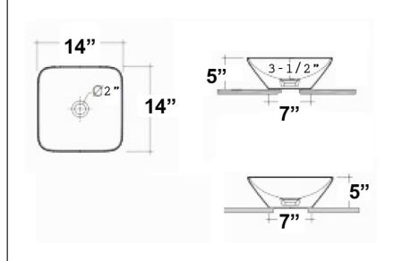
Dimensions of fixture are nominal and may vary within the range of tolerances established by AMSE Standard A112.19.2.2018 Dimensions and specifications subject to change without notice.
